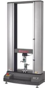
FMD/MMD Dual Column Motorized Test Stand
